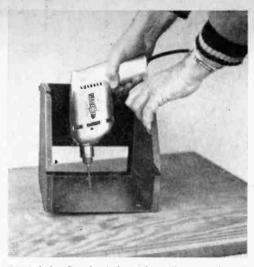
DRILL holes for the light socket. This must be set at a point to give equal lighting at the 4 holes.
