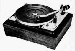
variations of 10%. The Dual 1009 has a variable speed control (6% variation) and has a built in switch which turns off the amplifier after play. Other features include: 4 speeds, 7 lb. non-ferrous turntable, interchangeable single play and changer spindles, continuous repeat, neutral gear, and slide switch controls. Specs for rumble, wow and flutter are claimed to match or surpass all professional caliber turntables. Price: \$94.75. (United Audio, 12 West 18th St., New York, N. Y. 10011)
