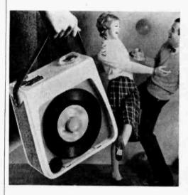
ture of permitting the record to be played while the unit is in any position, or even while it is being carried. The mechanism which accomplishes this trick includes a tone arm which plays from underneath the record (it contains a sapphire needle). Known as the "Swing Along," the unit is claimed to have what the manufacturer calls "remarkably big audio." The unit weighs 6 lbs., operates from four D batteries. Price: \$79.95. (Channel Master, Ellenville, N. Y.)
