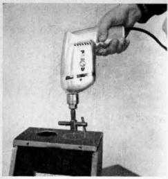
EXPANSION BIT is ideal for cutting the holes for the 4 different types of glass used in Meter Maid.
